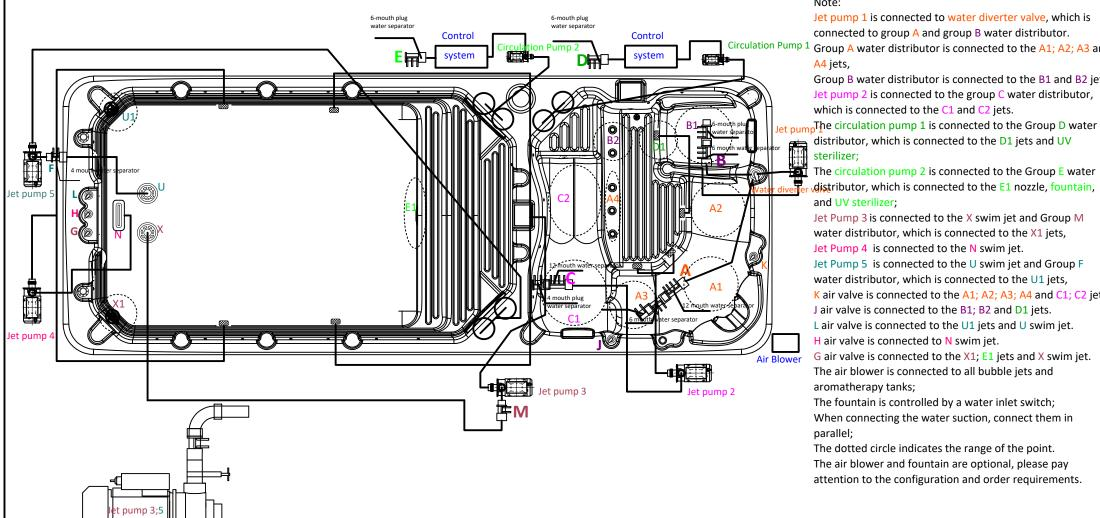
Note: Jet pumps 3 and 5 need to be placed vertically when installing the water distributor.
